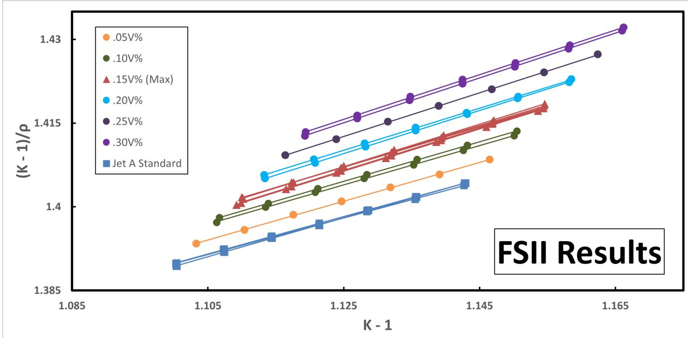
FSII measurably impacted the gauging slope across all concentrations and all temperatures tested. Gauging slope **b** linearly varies from 0.3475 to 0.4019.
